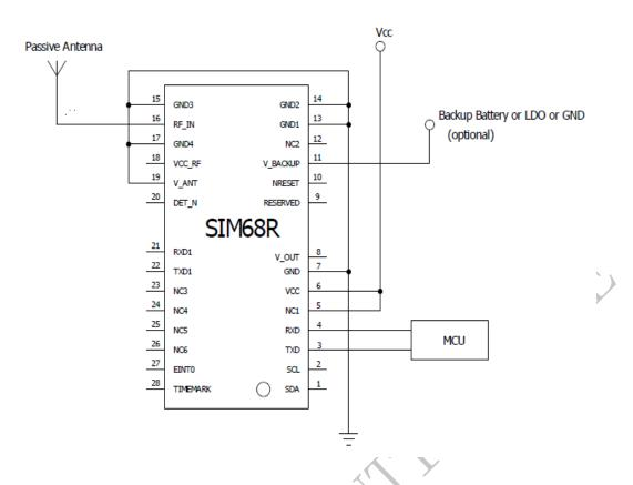
Figure 5: SIM68R passive antenna design
