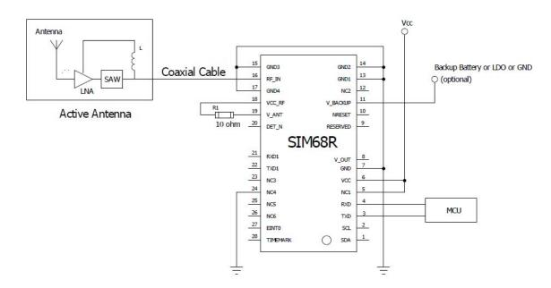
Figure 8: SIM68R Active antenna design
