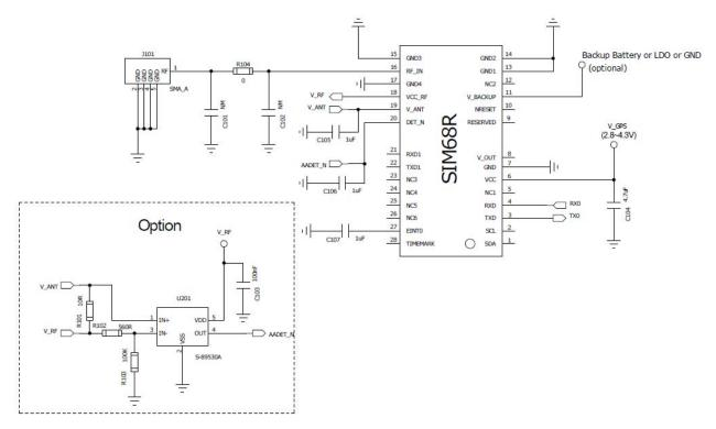
NOTE: the standard firmware does not support active antenna detection)
