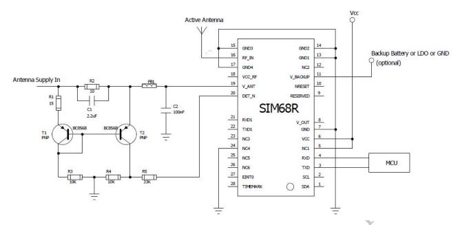
Figure 12: Open circuir detection-B
