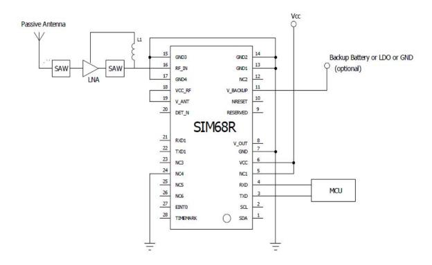
Figure 7: SIM68R passive antenna design for best performance
