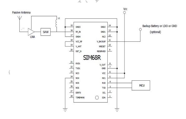
Figure 6: SIM68R passive antenna design (with external LNA and SAW)
