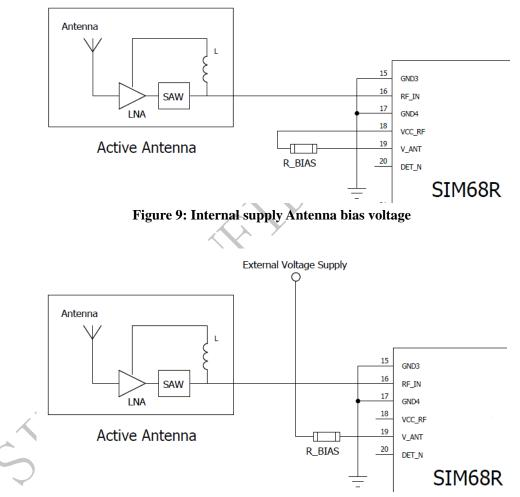
Figure 10: External supply Antenna bias voltage
